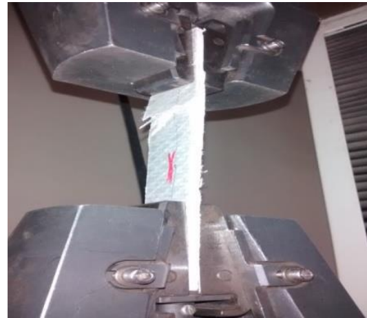
Fig. 5: Tensile test of GFRP laminate
