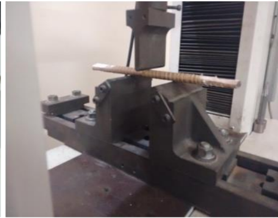
Fig 2: Flexure test of GFRP bar
